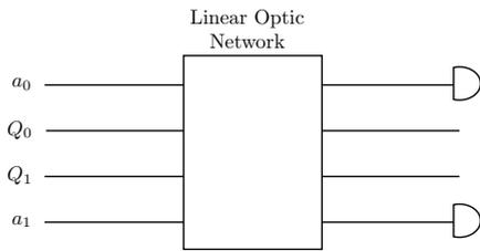
(a) Simplified diagram of a CNOT logic gate linear optic implementation where  $Q_0$  and  $Q_1$  represent the control qubit and the target qubit and  $a_0, a_1$  are two ancillary photons.
