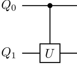
Fig. 3: The CU (controlled-U) logic gate.
