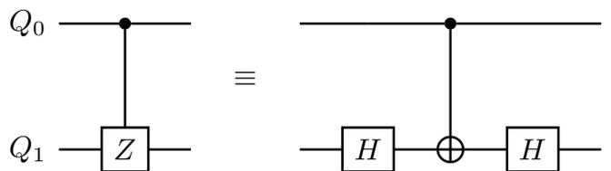
Fig. 6: Example of equivalent quantum circuit for a CZ logic gate exploiting the CNOT logic gate implementation.
