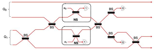
(b) KLM CNOT scheme with simplified NS gates.  $Q_0$  and  $Q_1$  denote the control qubit and the target qubit, respectively. This scheme assumes the logical qubits to be encoded through spatial modes (path encoding).
