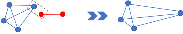
Fig. 8: Replace one node in C_4^3 state with a new qubit located at remote node. (1) A pair of EPR state is distributed among replaced and target nodes. (2) Performing Bell measurement on replaced qubit with one of qubit in given EPR state at the replaced node. (3) Replacing new node into C^4 state.
