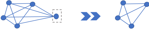
Fig. 6: Deleting one qubit from C_5^3 to C_4^3 . Performing Z-basis quantum measurement (denoted by dash rectangular) on the target qubit (solid blue dot surrounded by dash rectangular), while remaining qubits maintains C_4^3 state.
