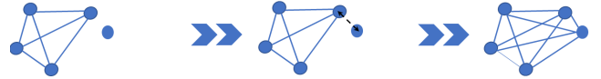
Fig. 3: Adding local qubit from C_4^3 to C_5^3 state. (1) New qubit (denoted in blue solid dot without link) is located at the same quantum node with an arbitrary qubit in C_4^3 state. (2) Performing CU operation, denoted as a black dash bidirectional arrow, on the new qubit with same located qubit. (3) Obtaining C_5^3 state denoted by 5-vertex full-connected graph.
