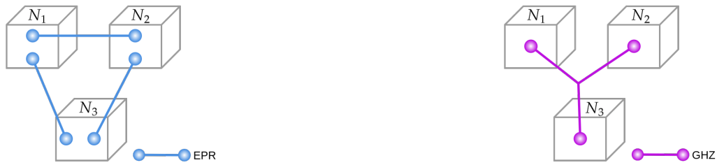
(a) EPR-based connectivity. For directly interconnecting three nodes, a minimum of three EPR pairs must be generated and distributed through the network. Once distributed, each EPR establishes a virtual quantum link between a fixed pair of nodes, namely, the nodes storing a member of the EPR pair.
